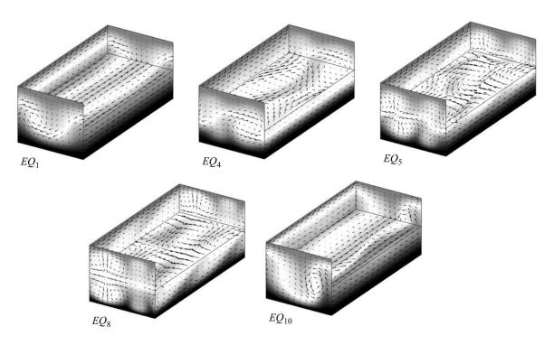
Figure 6: Equilibrium solutions of plane Couette flow in a  $2\pi/1.14 \times 2 \times 2\pi/2.5$  domain at Re = 400. The greyscale indicates the streamwise velocity of the fluid: light (dark) grey shows fluid moving at u = +1 (u = -1). Arrows indicate in-plane velocity. The top half of the fluid is cut away to show the (u, w) velocity in the y = 0 midplane. Note that solution  $EQ_1$  is a lower branch Nagata solution. After Gibson  $et\ al.\ [4]$ .
