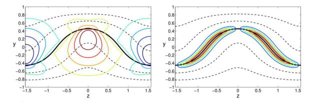
Figure 5: Representation of the solution studied by Wang et al. at Re = 50171. In both panels, the (black) open lines denotes contours of  $u_0$ , the thick line being  $u_0 = 0$ . The left (right) panel represents the contours of  $v_0$  ( $v_1$ ). After Wang et al. [21].
