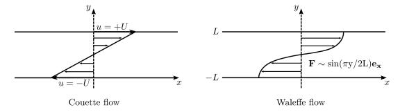
Figure 1: Sketch of plane Couette and Waleffe flows. Plane Couette flow is driven by wall motion in the x direction, the top and bottom walls moving with opposite velocities  $\pm U$ . Plane Waleffe flow is driven by a volume force in the x direction. The forcing is half a sine period in the y coordinate. Note that the laminar flow is stable despite the presence of an inflection point owing to the proximity of free-slip walls.
