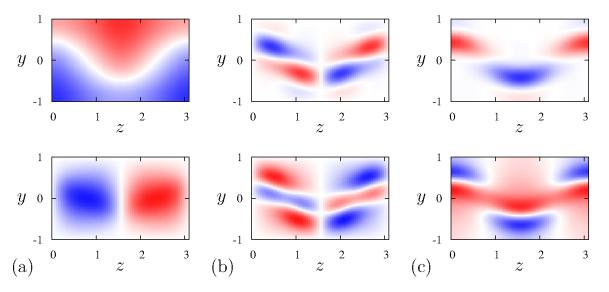
Figure 12: Flow fields at the last iteration for A=6.55 (see figure 11). (a) Top:  $\overline{u}^0$ , bottom:  $\overline{\psi_1}^0$ . (b) Top:  $\mathcal{R}(v_1')$ , bottom:  $\mathcal{I}(v_1')$ . (c) Top:  $\mathcal{R}(w_1')$ , bottom:  $\mathcal{I}(w_1')$ . In all cases, blue (red) represents negative (positive) values of the field.
