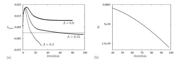
Figure 11: (a) Plot of the leading real eigenvalue  $\lambda_{max}$  as a function of the iteration for different amplitudes of the fluctuations. The horizontal line indicates  $\lambda_{max} = 0$ . Only the curve for A = 6.6 is stopped at convergence, that for A = 6.5 goes way below  $\lambda_{max} = 0$  and that at A = 6.55 converges very slowly. (b) Evolution of the difference E between two successive iterates of  $\lambda_{max}$  for A = 6.55 on logarithmic scale.
