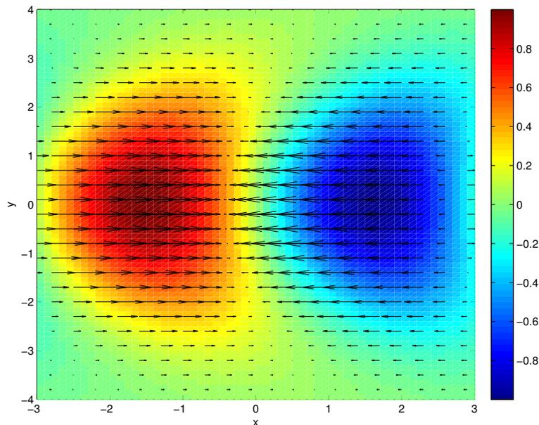
Figure 3: Pressure (surface height) in contours with overlay of the zonal velocity  $u$  field in arrows, for the “Kelvin”-like solution, for which  $|\omega| < N$ . The values for the constants are  $k = 1$ ,  $\ell = 1$ ,  $\beta = 1$ ,  $N = 3$  and  $2\Omega = 1$ .
