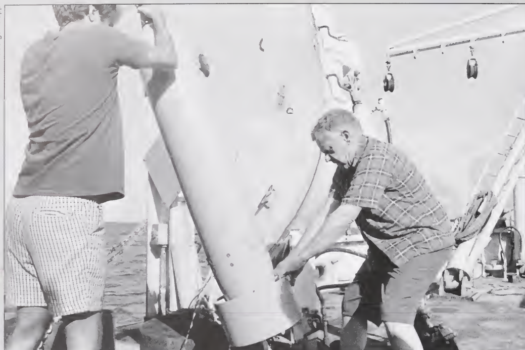
Hank helps Dave Bitterman manhandle a velocity-sensing tow body aboard Atlantis II in 1979.
