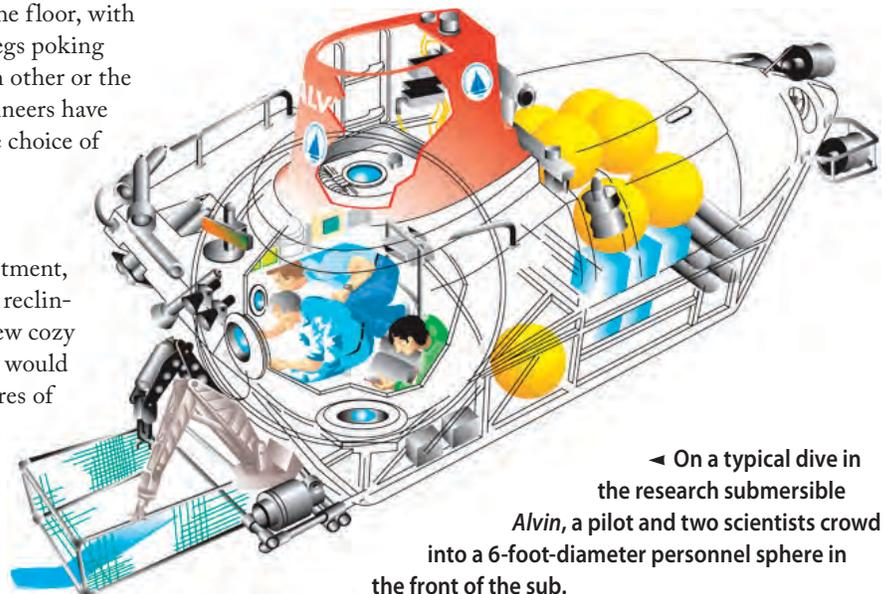
◀ On a typical dive in the research submersible *Alvin*, a pilot and two scientists crowd into a 6-foot-diameter personnel sphere in the front of the sub.
