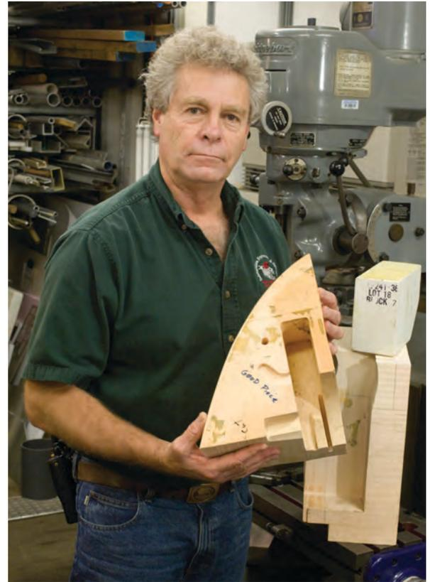
▲ WHOI engineer Rod Catanach is overseeing the development of new syntactic foam, the material used to provide buoyancy that allows *Alvin* to float back to the surface. The foam is made of a matrix of billions of microscopic hollow glass spheres embedded in a hard epoxy. It must withstand the crushing pressure at depths of 6,500 meters, or 4 miles.
