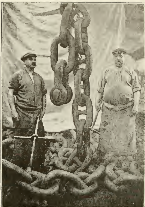
Anchor chains of the type used on the Titanic . Each link weighed 175 pounds. (Photo courtesy Ken Marschall collection: from The Largest Ships of the World , 1914)
