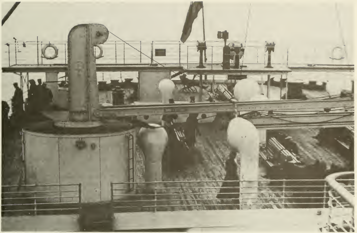
The poop deck of the Titanic (see also stern photo on pullout). Picture was taken while at Queenstown, Ireland. The baggage/freight handling cranes could each lift a maximum of 2½ tons. Note the two docking telegraphs on aft bridge and the one spotted in the debris field on page 28 (lower photo). (Photo courtesy The Cork Examiner)
