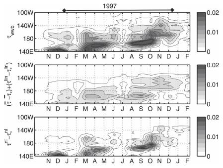
FIG. 4. (top) Average zonal wind stress over 5°N to 5°S due to WWBs,  $\tau_{WWB}$ . (middle) Part of the WWB zonal wind stress explained by the seasonal climatology and a linear response to SST,  $(\bar{\tau} - \bar{\tau}_*) + (\tau^{\text{lin}} - \tau_*^{\text{lin}})$ . (bottom) Part of WWB zonal wind stress unexplained by a linear response to SST,  $(\tau^{n1} - \tau_*^{n1})$ .
