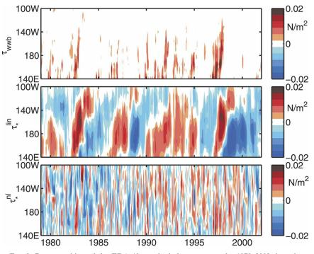
FIG. 3. Decomposition of the ERA-40 zonal wind stress anomaly, 1979–2002, into three components using the same format as in Fig. 1. (top) The WWB component of the winds. (middle) The non-WWB part of the wind stress is explained by the first seven singular vectors of an SVD analysis of the SST-wind stress covariance matrix. (bottom) The residual winds that are neither classified as a WWB nor explainable in the SVD analysis.
