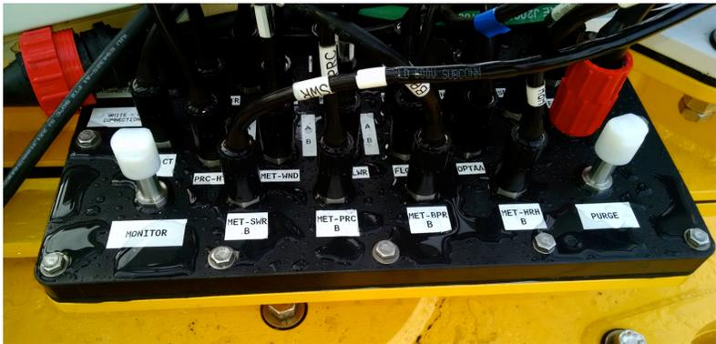
Figure 7: Monitor and Purge Ports
