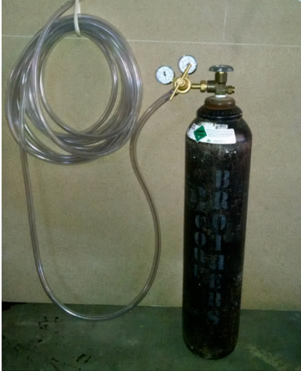
Figure 5: Nitrogen Tank, Regulator and Flexible Tubing
