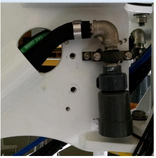
Figure 9: Vent Valve to be removed
