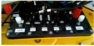
Figure 7: Monitor and Purge Ports
