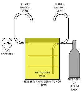
Figure 8: Instrument well purge procedure setup
