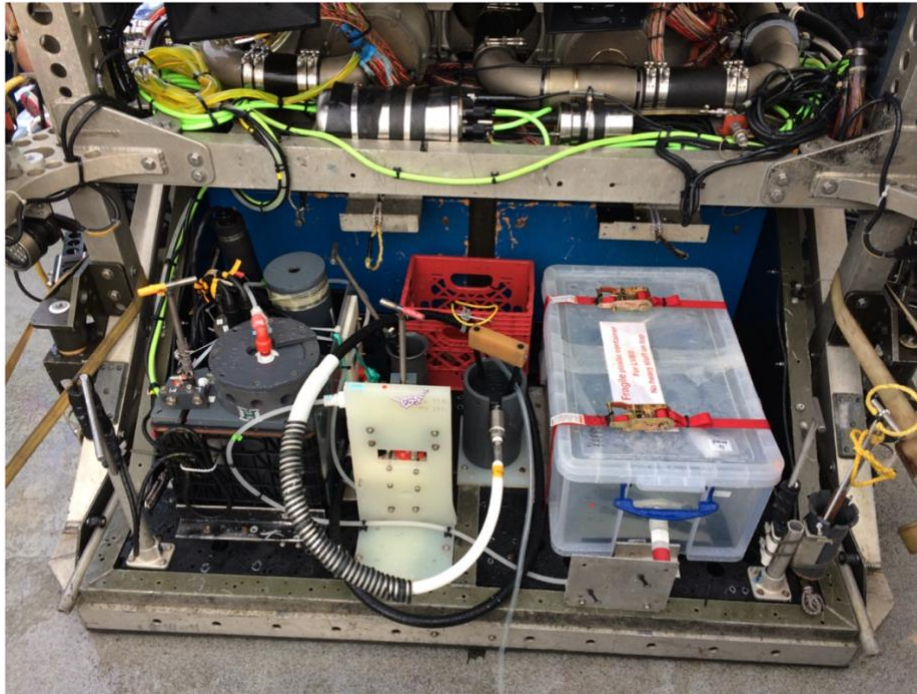
Figure 6. Mobile Pumping System (MPS) Controller and Large Volume Bag Sampler (LVBS). Top: Example of MPS (right and center) and LVBS (right) mounted on the front of Jason on dive J2-1024. Bottom: Schematic illustrating the connection of the MPS controller to the Jason junction box and peripheral sampling devices. See dive J2-1024 – J2-1028 config files for more information.
