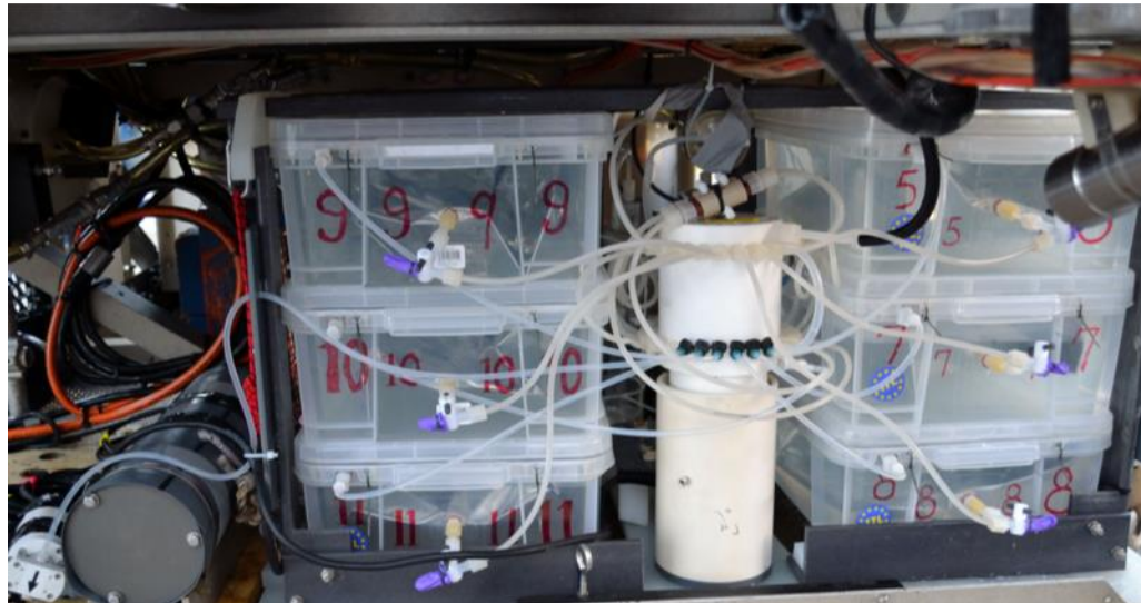
Figure 7. Medium Volume Bag Sampler (MVBS). Top: MVBS with McClane controller (left) and 24-port McClane manifold on skid mounted in back of Jason science sled on dives J2-1024 – J2-1028. Bottom: schematic illustrating the connection of the MVBS to the Jason junction box and MPS. See dive J2-1024 – J2-1028 config files for more information.
