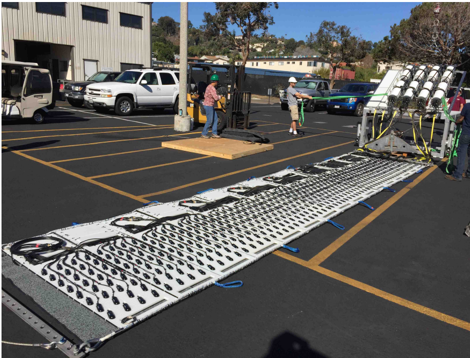
Figure 3. Physical configuration of the 512-element mid-frequency array arranged in a 2D distribution of elements (8 vertical staves of 64-elements each). Data acquisition electronics and battery pressure cases on top.
