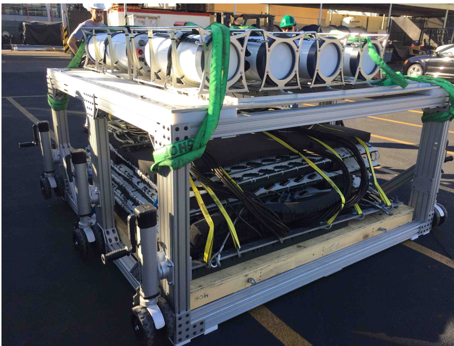
Figure 4. Cart for positioning of the 2D mid-frequency array on deck prior to deployment.
