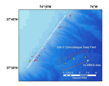
Site 2 Closeup of (Chincoteague) in the red survey box. The large yellow circles are new seeps found by the USGS (westerly ones) and by Skarke (easterly) aboard the R/V Atlantis SeepC cruise in 2015. The small vellow dots and the red/green dots on the upper slope are from our 2014 Nature Geoscience northern Atlantic margin database of plumes. mapped with water column backscatter from the NOAA OER EM302.
