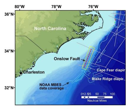
Survey along the strike of the fault: 70 nm or ~9 hours for MBES/EK80 collected at 8 knots. This will provide a severalkm-wide swath and backscatter directly along the fault.
