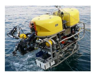
The K2 platform uses a dual tether, down-weight system, comprised of a main 1220 meter electro-optic, strength (Kevlar) reinforced umbilical spooled on an oceanographic winch that is coupled to a secondary 45 meter electro-optic flying tether. A variable weight depressor frame, configured between 500-1000 pounds, provides a junction point for this transition as well as isolation between the vehicle's movements and those of the support vessel above.
