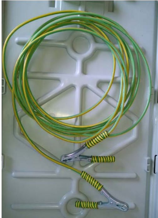
Figure 4: ESD Ground Strap
