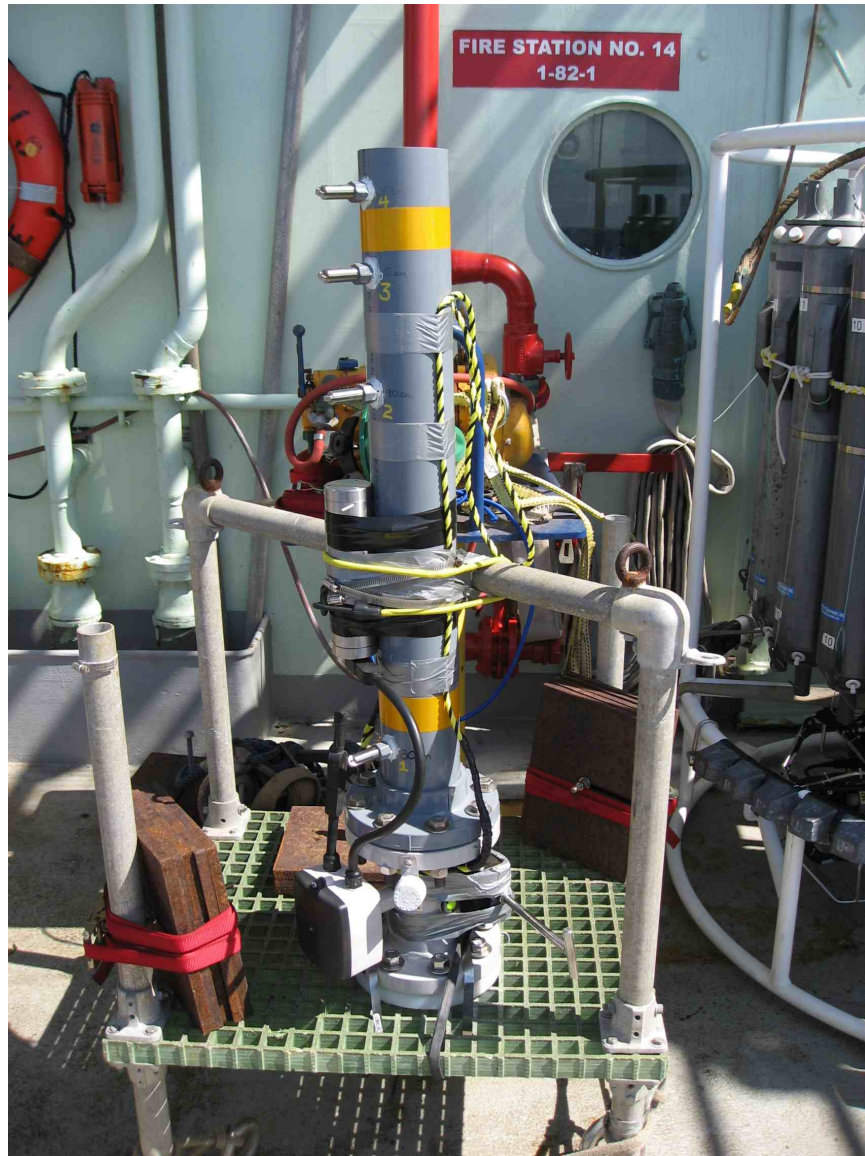
Figure 1. Small ("Alvin") elevator used over the side during Atlantis/Jason expedition AT18-07 in Summer 2011. The elevator is figured in this photo for calibration of an electromagnetic flowmeter. The grating on this elevator was cut near the center, to make room for a plastic adapter that extends through the grating and holds the flowmeter securely in place, allowing water to move freely up/down through the flowmeter. We lowered and raised the flowmeter on the hydrowire, as an over-the-side night operation, to calibrate the flowmeter. After this, the flowmeter was deployed on a CORK wellhead, where it currently resides. This flowmeter will be recovered in Summer 2013, and may be redeployed on a different wellhead. We would like to calibrate a second flowmeter, and may wish to recalibrate this flowmeter, depending on the nature of data recovered in Summer 2013.
