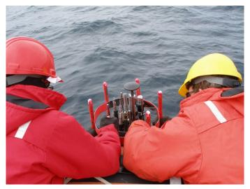
ASIP is lifted over the side of the RHIB and the sensor cover is removed before release
