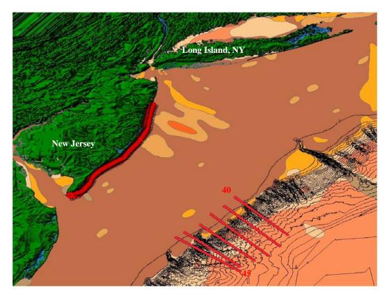
Figure 1. Transects along the New Jersey coastline in which submarine landslides pose an elevated tsunami hazard (up to 4-m of inundation for a 500-year tsunami event).
