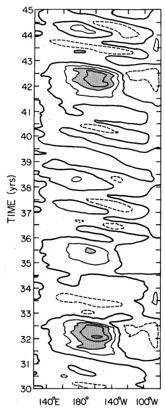
FIG. 13. Equatorial zonal wind stress anomalies between year 30 and year 45 of the model simulation. Positive (westerly) anomalies are indicated with solid lines, and negative (easterly) anomalies are indicated with dashed lines. Large westerly anomalies ( $\geq 0.15$  dyn/cm<sup>-2</sup>) are stippled.
