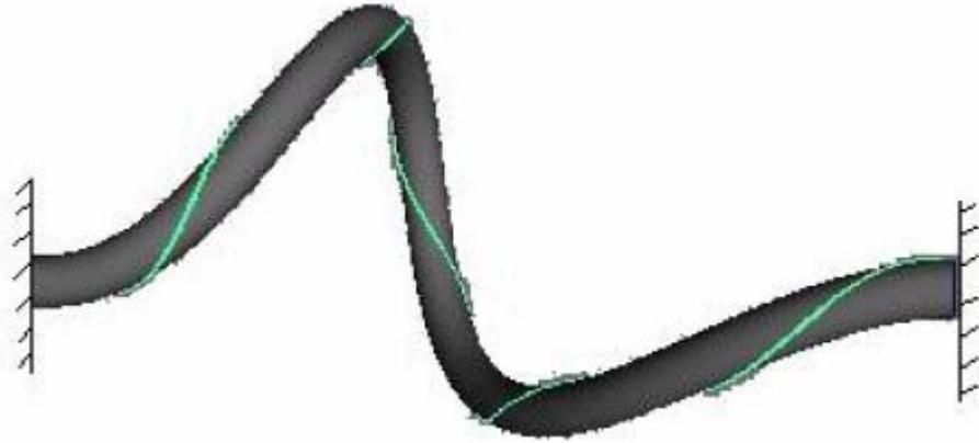
**Figure 4.1 Benchmark problem: a twisted and clamped rod. The ends have prescribed twist and separation.**
