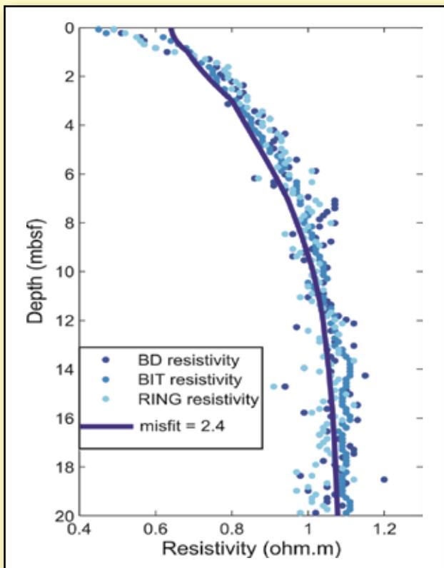
◀ An example of a resistivity profile (blue line) derived from inverting data from the EM System in the Gulf of Mexico (1,300 meters water depth). Blue dots are measurements made during adjacent drilling operations.
