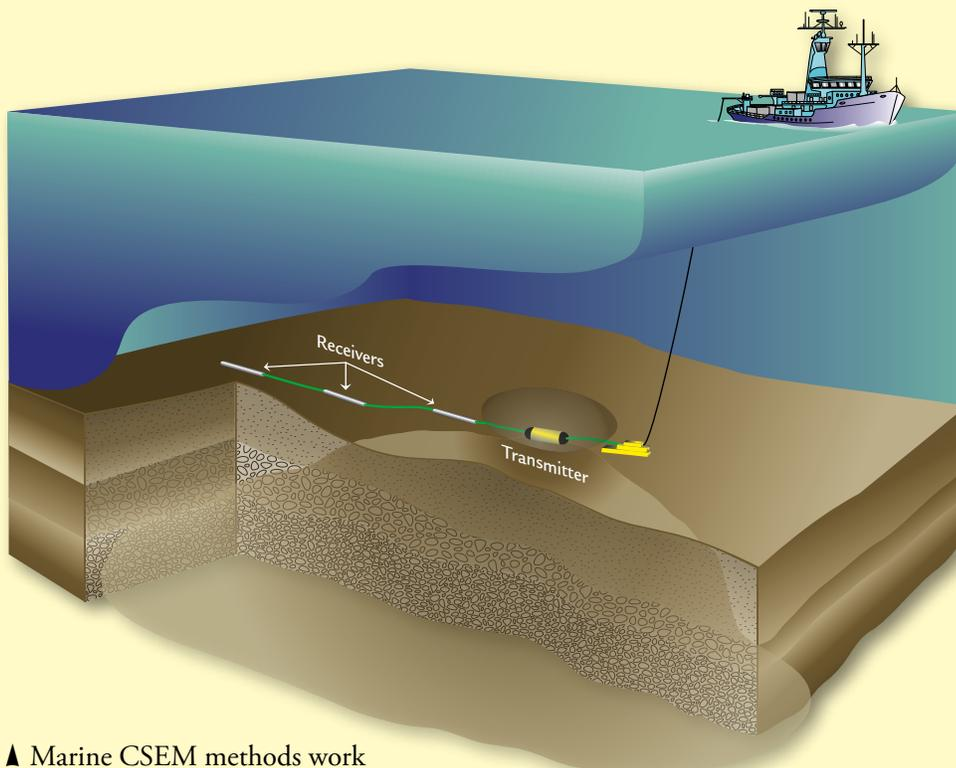
▲ Marine CSEM methods work by transmitting harmonic magnetic fields that decay with distance according to the skin depth of the media. The fields decay more rapidly in the more conductive seawater than in the subseafloor, making measured fields more sensitive to sub-bottom structure than conventional DC resistivity methods. Unlike other large scale CSEM methods, our system is a profiling tool that can be used to make maps of surficial properties.
