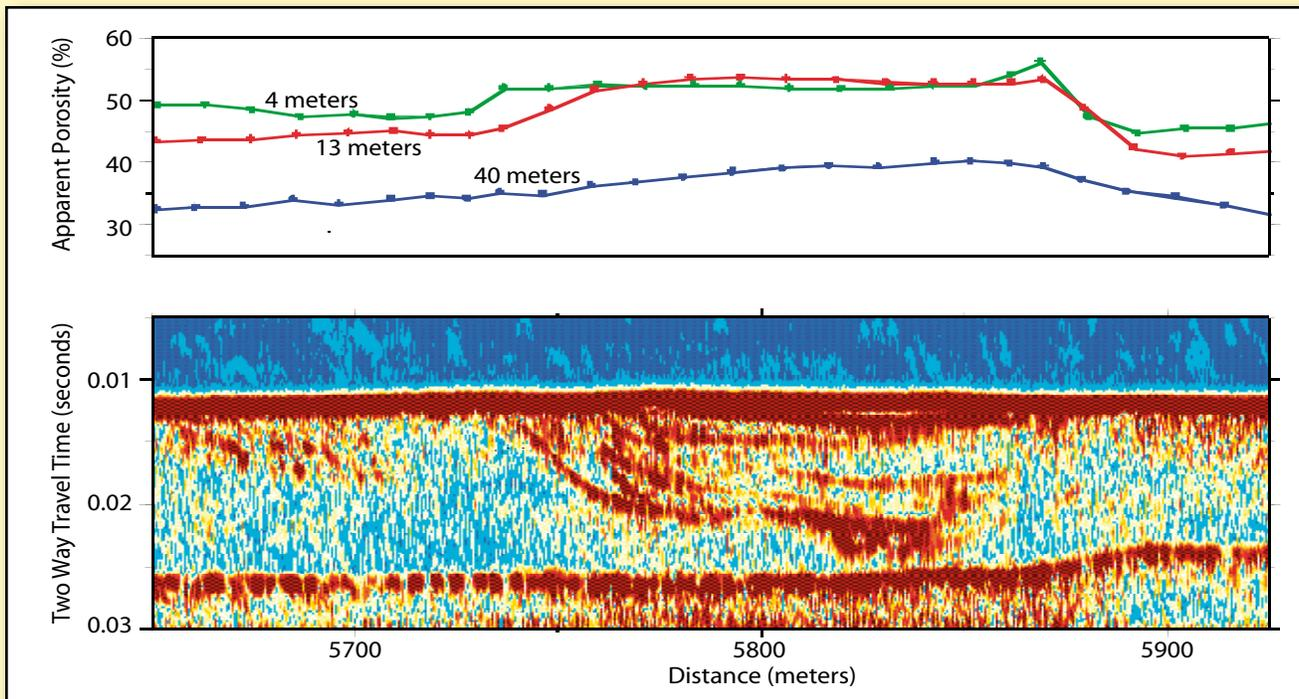
▲ An example of data collected by the WHOI EM System, off North Carolina. Top panel shows raw data from the system displayed as apparent porosities, one profile for each of the three receivers. In the figure the green symbols are the porosities measured by the 4 meter receiver which senses over the top 2 meters of
