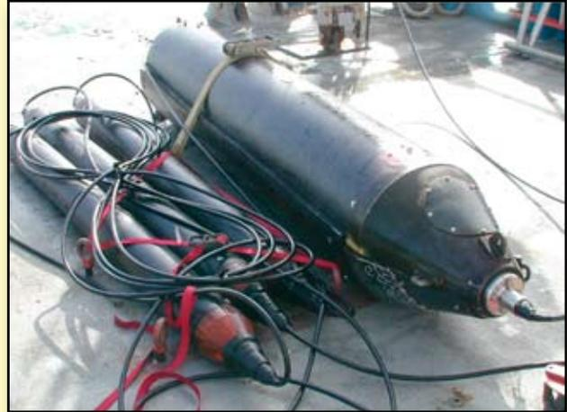
▲ A photograph of the towed EM system on deck. The system consists of a transmitter (large cylinder) connected to the ship by a 0.680 conducting cable.
