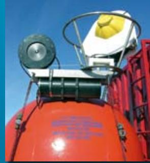
An upward-looking sonar measures the thickness of ice flowing over the mooring.
