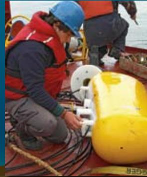
An acoustic Doppler current profiler uses sound waves to measure current speeds and directions.
