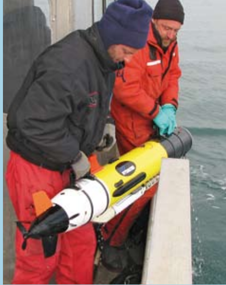
A WHOI engineers Greg Packard (right) and Jeff Lord deploy a REMUS underwater vehicle off Barrow, Alaska, where the formation of sea ice “transforms” waters from the Pacific and makes them saltier and denser.
