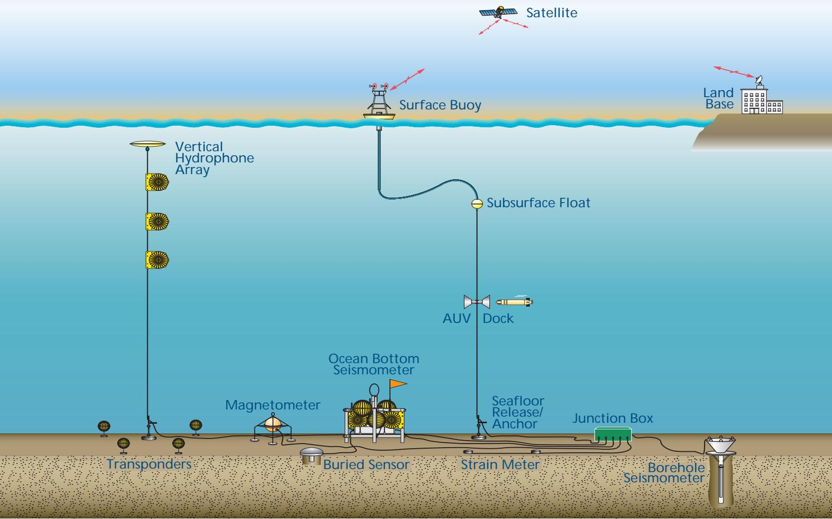
syntactic material to support the weight of 3,000 meters of cable. A fluid-filled, stretchable rubber hose with an integral coil of electrical conductors would connect the subsurface and surface floats. By carefully distributing flotation along the upper cable section, we can maintain an “S”-shaped tether to effectively isolate the subsurface float from the motion of the surface buoy.
