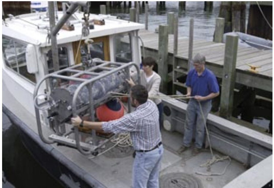
SHORE TO SHIP—WHOI researchers Alexi Shalapyonok, Heidi Sosik, and Robert Olson (left to right) carefully load the FlowCytobot onto a WHOI research vessel for installation on the seafloor at the Martha's Vineyard Coastal Observatory. The instrument counts and identifies protist cells in the water, and the data is transmitted via undersea cable back to shore.
