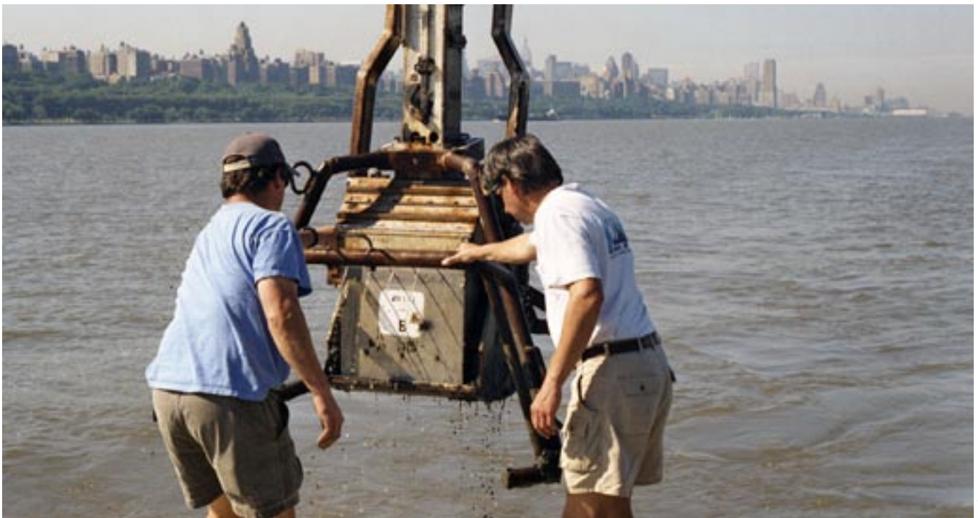
MIXING IT UP IN GOTHAM—WHOI Senior Research Assistant Jay Sisson (left) and Engineer Craig Marquette maneuver a box corer after plucking a 30-centimeter-deep sample of sediment from the bottom of the Hudson River in June 2001. Within sight of Manhattan, the researchers measured the rate at which sediment accumulates along this intersection between salty ocean water and fresh river water.
