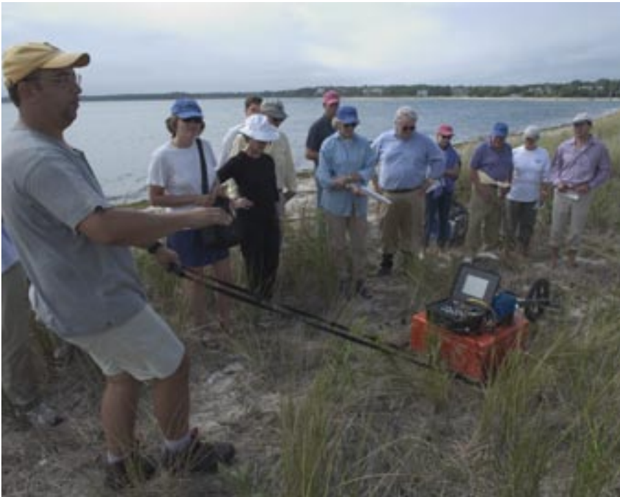
WHOI Assistant Scientist Ilya Buynevich demonstrates the use of a ground-penetrating radar instrument on a beach in Cotuit, Mass. By bouncing radar waves off buried rocks and sediments, he can create maps of subterranean layers and extrapolate sea level in years past.
