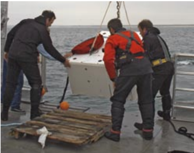
UNDERWATER POWER STRIP —Left: The seafloor node of the Martha's Vineyard Coastal Observatory, shown here being lowered into the water, supports experiments but it is also an experimental technology itself. Scientists plug into the node's power supply and data cables to study everything from shifting sands to blooming plankton. Right: New robotic technologies and cutting-edge instruments—such as the plankton-observing FlowCytobot—are tested at MVCO before heading off to projects in other regions.
