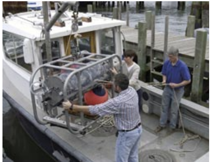
UNDERWATER POWER STRIP —Left: The seafloor node of the Martha's Vineyard Coastal Observatory, shown here being lowered into the water, supports experiments but it is also an experimental technology itself. Scientists plug into the node's power supply and data cables to study everything from shifting sands to blooming plankton. Right: New robotic technologies and cutting-edge instruments—such as the plankton-observing FlowCytobot—are tested at MVCO before heading off to projects in other regions.
