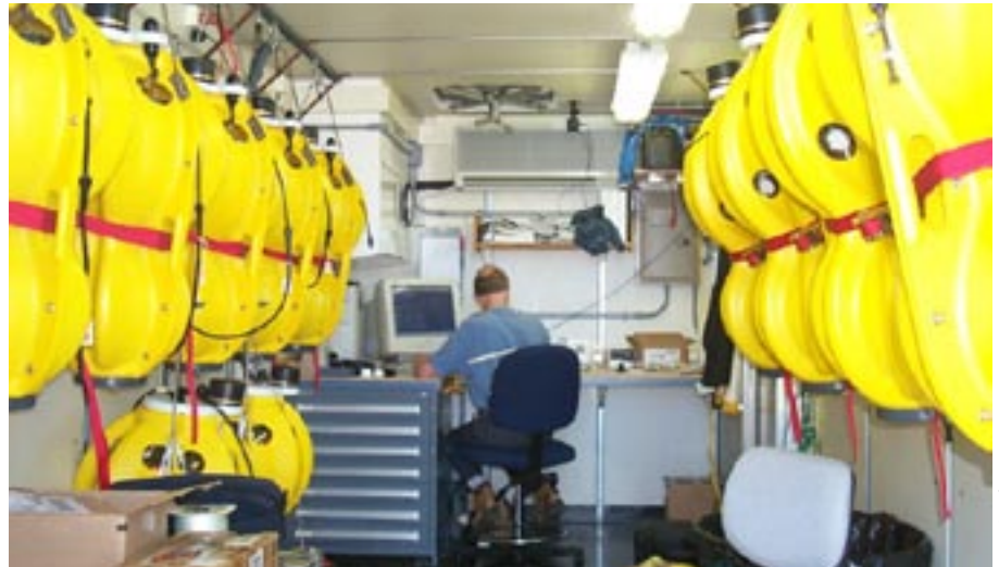
A vanload of new WHOI "D2" ocean-bottom seismographs is readied for field testing. The D2s are small and light, for easy deployment and recovery. With a six-month battery capacity, they are designed for relatively short-term experiments. The D2s are available to scientists through the newly created National Ocean-Bottom Seismograph Instrumentation Pool. WHOI Senior Engineer Ken Peal, who helped design the D2, is in the background.
