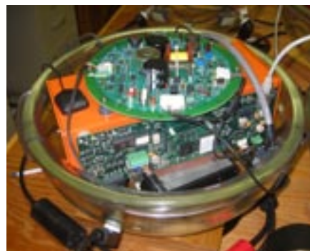
The D2's electronic data logger (above), which records seismic wave measurements, resides in a glass ball in one half of the peanut-shaped D2. Batteries are in the other half.
