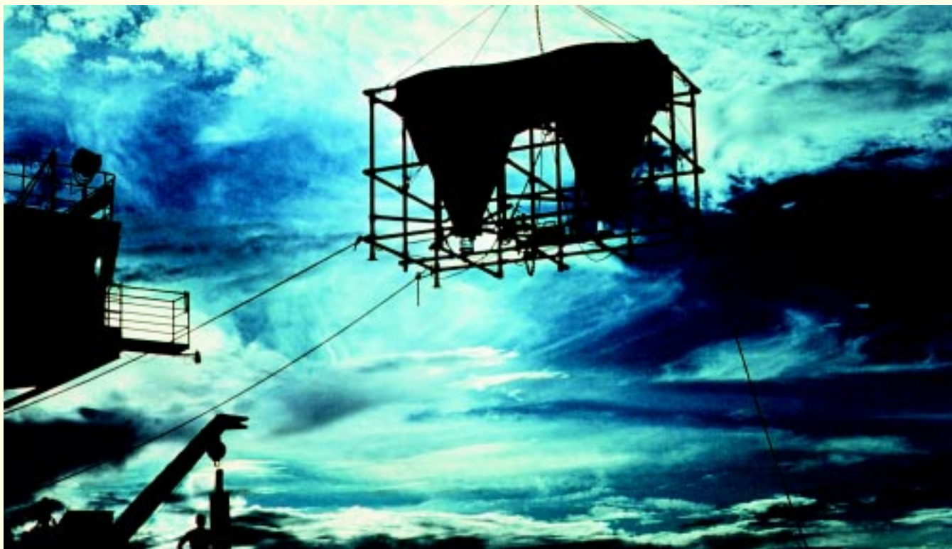
Honjo's early sediment traps were large, gray cones, often deployed in pairs.
