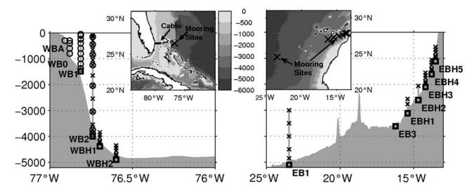
**Fig. 1.** Distribution of density (crosses) and bottom-pressure sensors (squares) of the RAPID/MOCHA moorings at the western and eastern boundaries of the subtropical North Atlantic near 26.5°N that are used for computing the zonally integrated meridional geostrophic flow. Direct current—meter measurements at the western boundary (circles)
