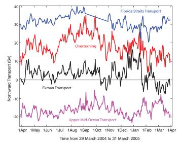
winds. The upper mid-ocean transport, based on the RAPID time series, is the vertical integral of the transport per unit depth down to the deepest northward velocity (~1100 m) on each day. Overturning transport is then the sum of the Florida Straits, Ekman, and upper mid-ocean transports and represents the maximum northward transport of upper-layer waters on each day (SOM text).
