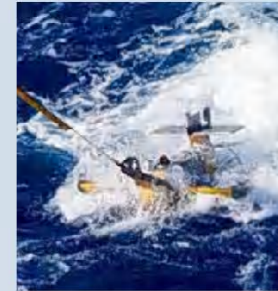
SeaSoar trawl measures properties of water up to 300m deep
