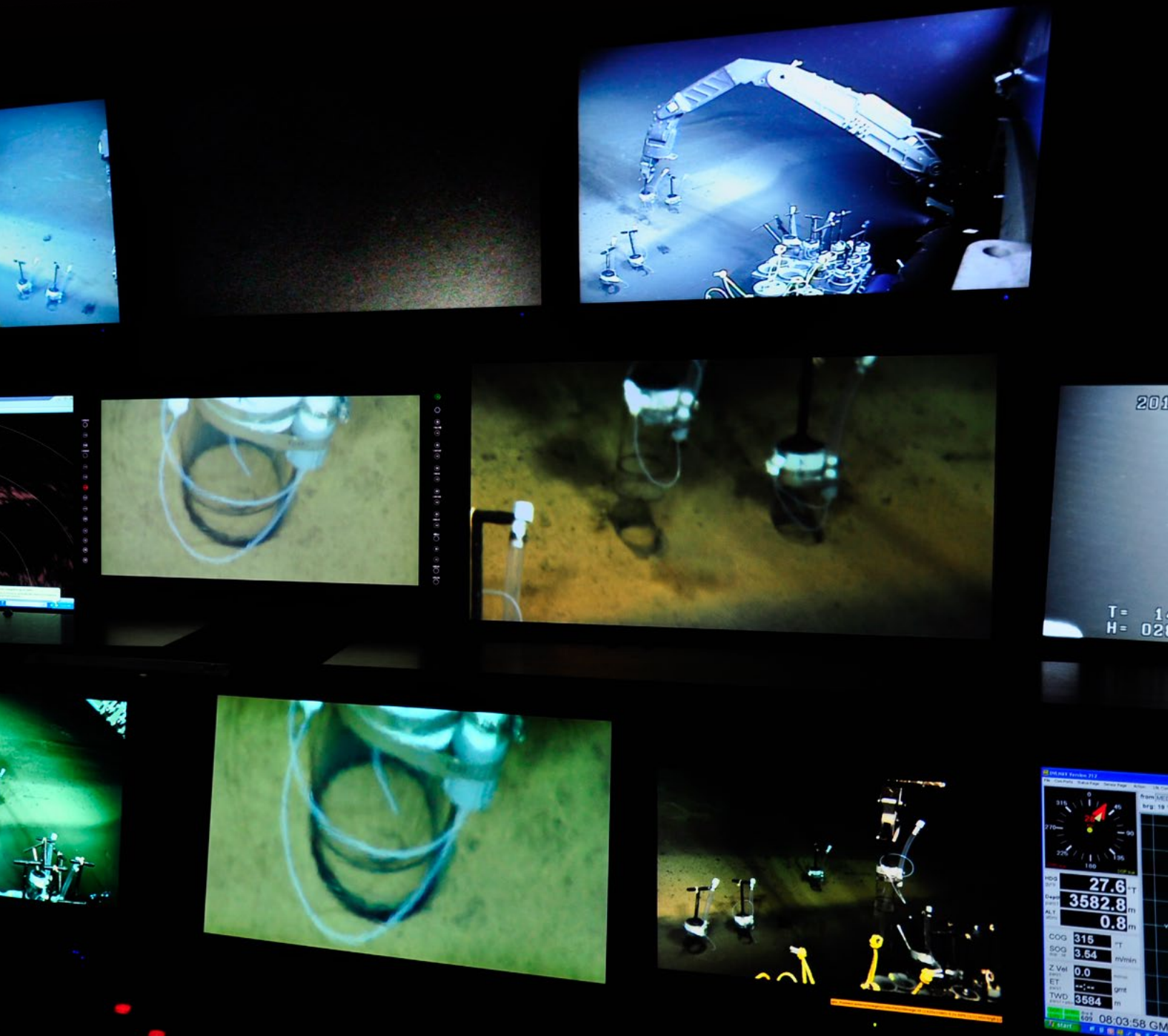
In the control van of the remotely operated vehicle Jason , pilot Tito Collasius (at left, in foreground) uses live feeds from several cameras to maneuver one of the vehicle's manipulator arms (upper right) to collect sediment samples from a DHAB and its white "beach."
