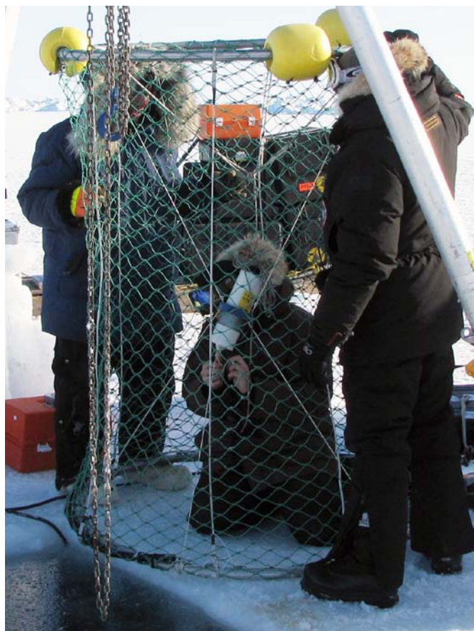
Fig. 4. Photo of the AUV capture net being prepared for deployment. Note the USBL homing beacon being suspended in the center of the net.
