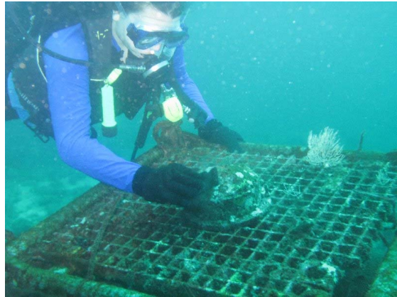
Plate 2. PLUTO node being readied for deployment (top left). Fiber optic ground cable being deployed from barge (top right). Connectors on node after 2 years in water (bottom left). Diver (A D York) cleaning the ADCP (bottom right).
