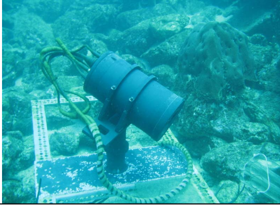
Figure 3. Pan and tilt camera installed at the PLUTO observatory. Note fish condos on the bottom right being observed by the camera. Water visibility during this time of year (April) was poor due to high levels of plankton. A red tide started blooming on April 8, 2008
