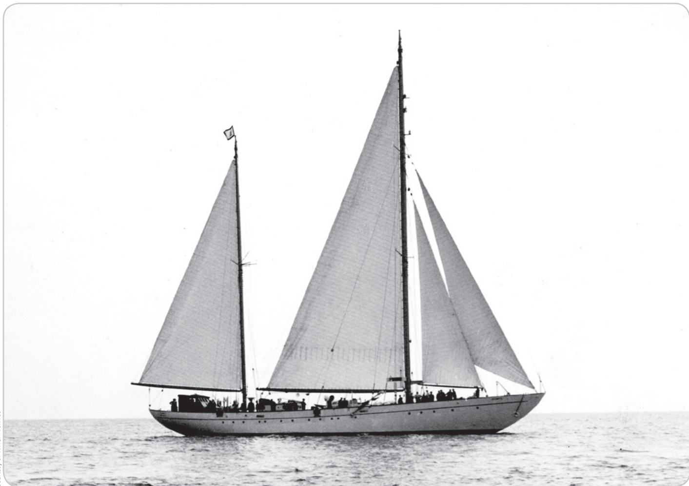
Built in 1931, Atlantis was WHOI's first ship. As the first vessel built specifically for deep-water oceanographic research, the 143-foot ketch rejuvenated the field, making 299 cruises until it was retired in 1964.
