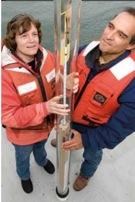
Oceanographers Amy Bower and David Fisichella hold a RAFOS float, which can drift for years in the oceans, recording locations and water conditions.
