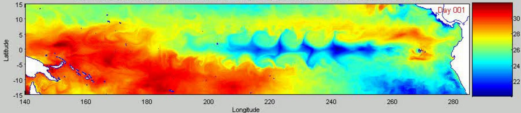
Tracer, EQPAC, year 1995. Tracer released at 95W, 1S-1N, top 10 meters. Time of release: April and September.
