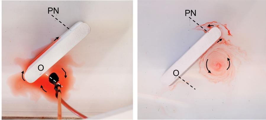
**Figure 14.** Top views of laboratory experiments for a baroclinic anticyclone (left panel) and a barotropic cyclone (right panel) impinging on a tilted island. Arrows indicate direction of flow. Dashed lines represent the O-line and PN-line as in Figure 12.
