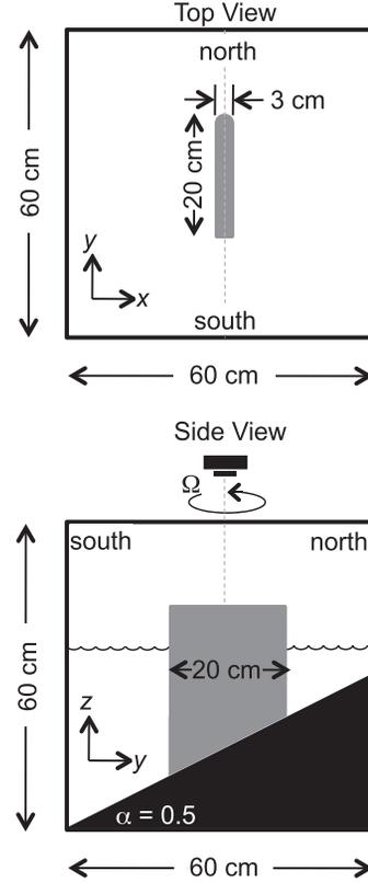
**Figure 4.** Experimental setup. Top view (upper panel) and side view (lower panel) showing the island (gray) and sloping bottom (black). Not to scale.
