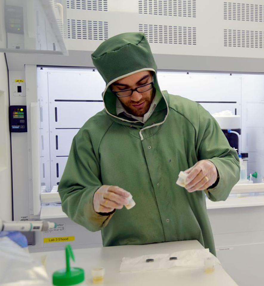
Top: Adam Sarafian prepares samples of meteorites to remove all contamination from the sample surface in the clean room in WHOI scientist Sune Nielsen's NIRVANA (Non-traditional Isotope Research on Various Advanced Novel Applications) lab.
