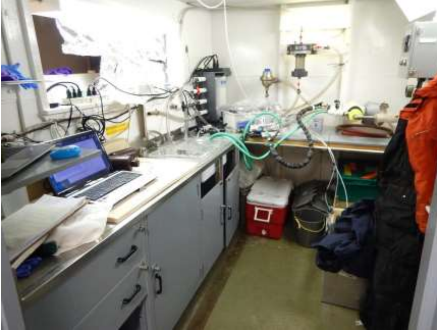
Figure 21. Seawater loop system – 2017 (similar for 2018)
