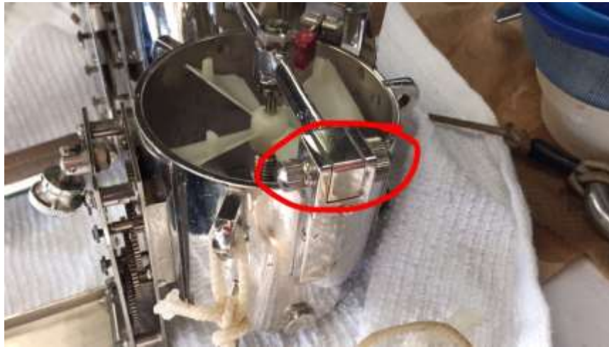
Figure 2. TSK flowmeter crossbar nut and bolt which came loose during the 2018 JOIS cruise.
