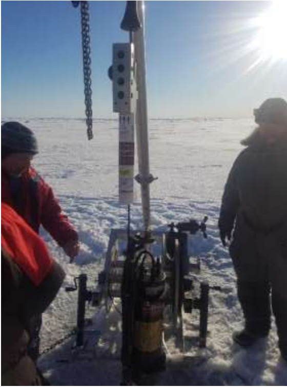
Figure 16. SAMI-CO 2 and Seabird Microcat w/ dissolved Oxygen deployed on ITP 110 during the first ITP deployment.
