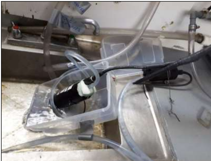
Figure 29. Outflow from Chl fluorometer feeds into the CDOM fluorometer sn1281. Barbettes added to CDOM sensor Sep 7 th .
