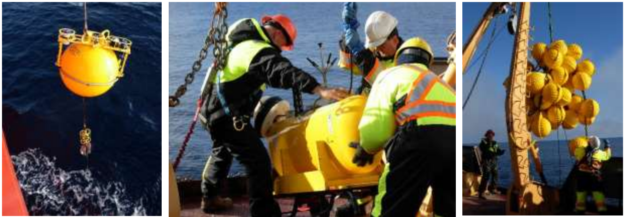
Figure 1. Recovery of top floatation package (left), MMP (center) and backup floatation cluster (right) of mooring D.
