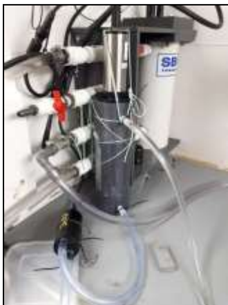
Figure 27. Outflow from Chl fluometer feeds into the CDOM "can" with fluorometer sn1076.
