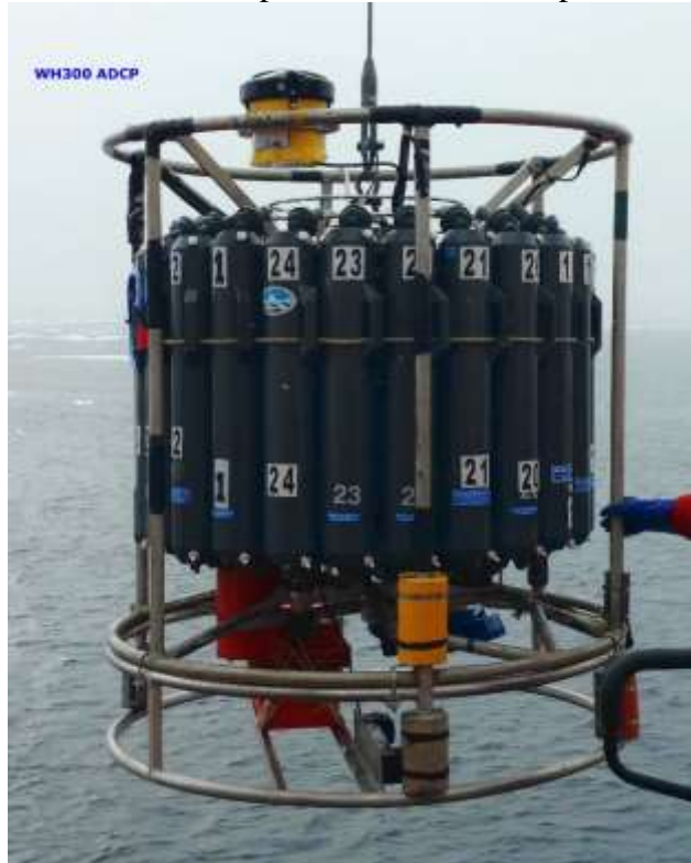
Figure 1. CTD Rosette with LADCP, FOGLogger, and Microrider (not all visible).
