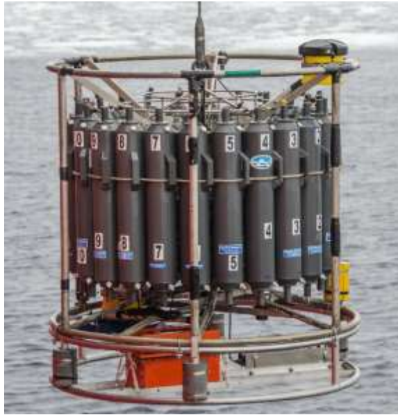
Figure 14. The rosette showing the addition of LADCPs and orange battery back. The CTD, FOG logger and Micro-rider are hidden by the Niskin bottles.
