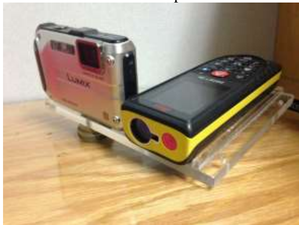
Distance meter and digital camera
