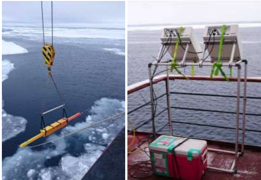
Figure 2 Pictures of EM and PMR installed on the starboard side of LSSL.
