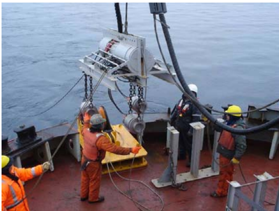
Figure 21. The tow sled being deployed.
