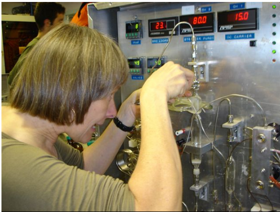
Figure 8. Nes Sutherland with the CFC sampling apparatus.
