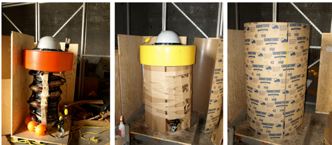
Figure B-3: Two restrained drifters are being prepared for deployment in the Keelung harbor warehouse. The cable is held in the correct deployment configuration with water soluble paper tape and cardboard board and tubes.
