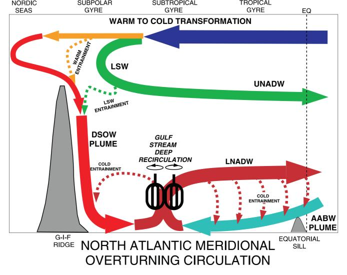
Figure 1. Schematic of the meridional overturning circulation of the North Atlantic Ocean, emphasizing the counterrotating deep recirculations of the Gulf Stream System acting to mix the convergent plumes of cold DSOW from the north and AABW from the south with overlying warmer deep waters to produce a homogeneous LNADW that dominates the deep water export from the North Atlantic.
