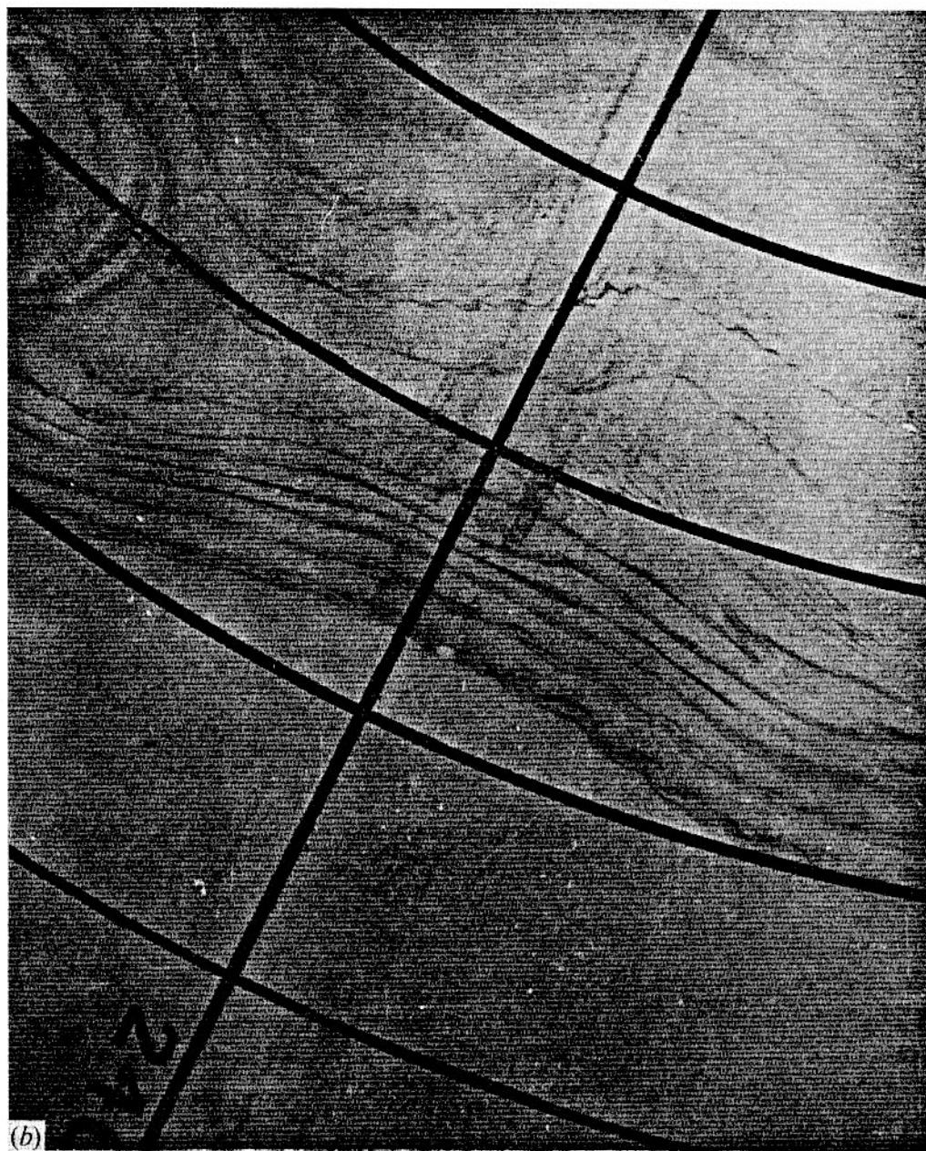
FIGURE 8. Experimental streamlines for \epsilon = 0.10 , b = 0.504 , E^{\frac{1}{2}} = 0.029 and h_0/\epsilon = 3.0 . (b) was taken at a slightly later time than (a), as the bump moved by beneath the camera, and thus shows more of the wake.
