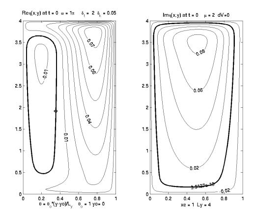
Figure 6. The real and imaginary parts of the solution for periodic forcing at frequency  $\omega = \pi$ . The parameter settings are otherwise as in Figure 2. The heavy lines are the zero contours of real and imaginary  $\eta$ .
