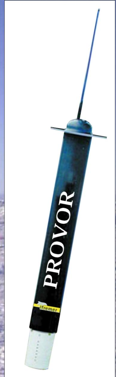
Both meteorological data and oceanographic profiling data acquisition are configurable. The power budget calculations indicate an expected life time of 24 months for hourly meteorological data acquisition with a position and CTD profile every 5 days.
