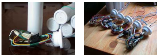
Figure 1a,b: Motorola MPX2200AP pressure sensors in hermetic vials equipped by two-cascade amplification microchip LM358 .
