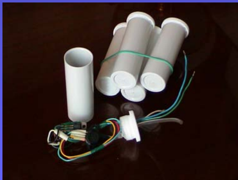
Figure 4.2: Pressure sensors with amplifier microchip in hermetic vials (front, opened).
