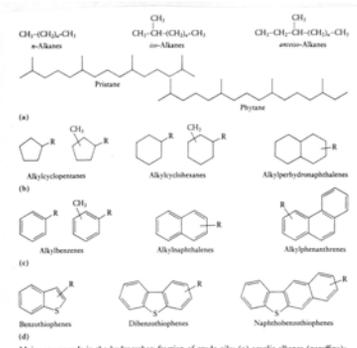
Major compounds in the hydrocarbon fraction of crude oils: (a) acyclic alkanes (paraffins); (b) cycloalkanes (naphthenes); (c) aromatic hydrocarbons; (d) sulphur-containing aromatics.
