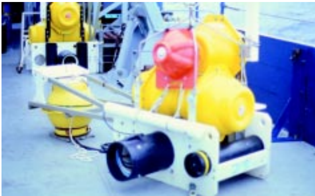
Figure 1. Webb OBS, one of the new generation of wide-band, long-deployment OBS that can be used in studies of the oceanic upper mantle. (photo courtesy of R. Detrick, WHOI)
